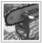
3. & 4. File cutter using gauge to ensure correct angle
